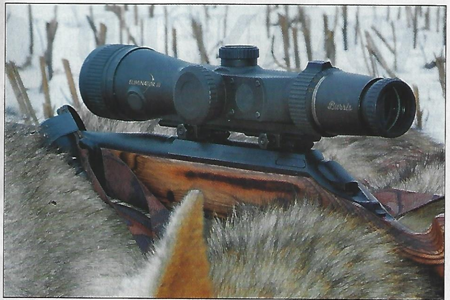
The Burris Eliminator III ranges the distance, and a lit red dot on the vertical wire (above) indicates the aim point.
